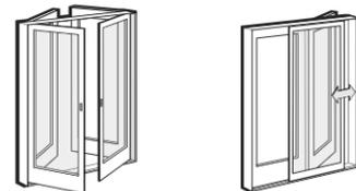
Single- or double-hinged insect screen for inswing single- and two-panel doors.
