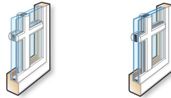
Permanent exterior and permanent interior with spacer
