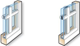
Permanent exterior and permanent interior with spacer
