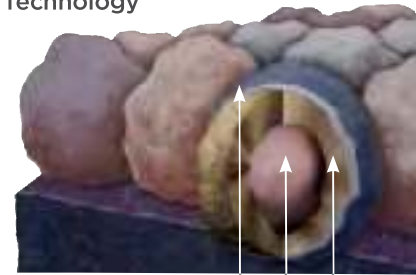
Ceramic coating Mineral core Copper layer Diagram for illustrative purposes only.
