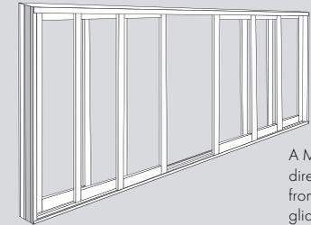
A Multi-Slide Door with a two-directional configuration opens from the center (like a bi-parting gliding patio door).
