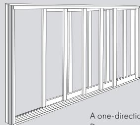
A one-direction MultiGlide™ Door can open from either the right or the left, and can either pocket or stack.
