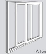
A two-panel gliding patio door has one moving and one non-moving (stationary) panel.
