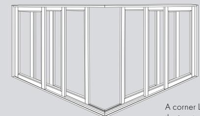
A corner Liftslide Door meets at the juncture of two walls for the most impressive opening and doesn't need a corner post!
