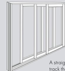
A straight Liftslide Door runs along a track that aligns with the wall. It can open from the right or the left and either stack or pocket when open.
