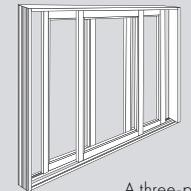
A three-panel gliding patio door has a stationary panel in the center, and moving panels on both the left and right.
